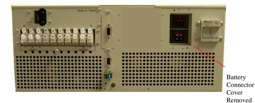
Once this has been done the battery cables supplied can be connected between battery connector on UPS and battery connector on each battery module. The cable supplied has a simple push fit Anderson connector at each end.
