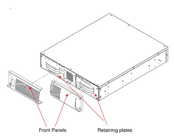
First remove both front panels as shown above. Then remove both retaining plates to gain access to the battery packs.
